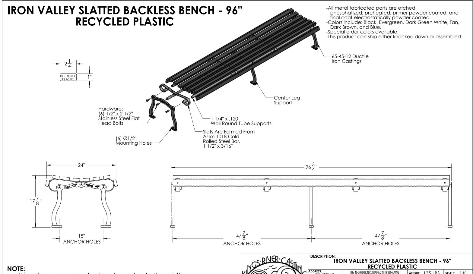
It is not recommended to locate anchor bolts until the bench is in place. Anchor bolts not included.
